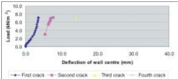
Fig 4. (left) Load vs deflection – grey wall
