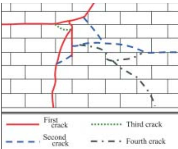
Fig 5. (left) Crack pattern – grey wall
