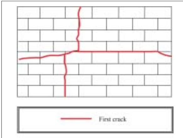
Fig 7. Crack pattern - yellow wall
