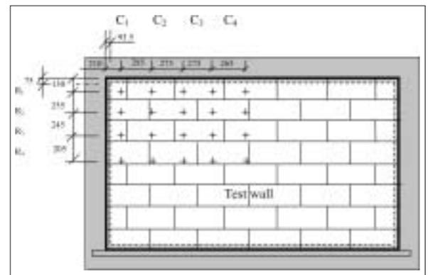
Fig 3. Yellow wall – location of LVDTs
